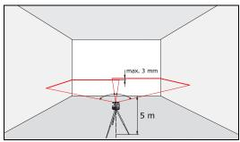
Set up the instrument on an even and flat surface. Allow the instrument to level.
