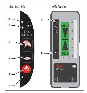
If the laser is in pairing mode and does not receive the signal from the remote, it will turn off after 30 seconds.
