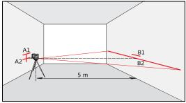
Then place the instrument at the same elevation as close as possible to wall A and again mark the horizontal laser line on wall A (-> A2). Rotate the instrument by 180° again and mark the laser on wall B (-> B2). Measure the distances of the marked points A1-A2 and B1-B2. Calculate the difference of the two measurements. If the difference does not exceed 2 mm, then the Leica Lino is within tolerance.
